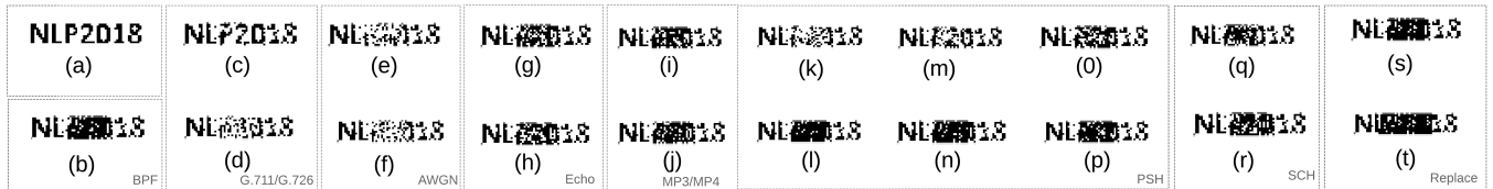
Fig. 5. Comparison of the watermark image between an original image (a) and the reconstructed images after performing the following signal-processing operations: (b) BPF, (c) G.711, (d) G.726, (e) AWGN (15 dB), (f) AWGN (40 dB), (g) Echo (20 ms), (h) Echo (100 ms), (i) MP3, (j) MP4, (k) PSH +20%, (l) PSH -20%, (m) PSH +10%, (n) PSH -10%, (o) PSH +4%, (p) PSH -4%, (q) SCH +4%, (r) SCH -4%, (s) Replace (1/3), and (t) Replace (1/2).
